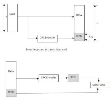
Error detection at receiver end
