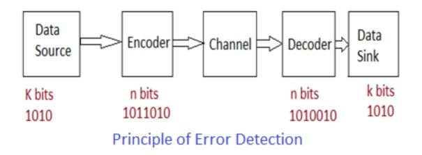
• When frame is transmitted from transmitter to the receiver. There are two possibilities viz. frame is received without error, frame is received in error (i.e. frame is bad).
